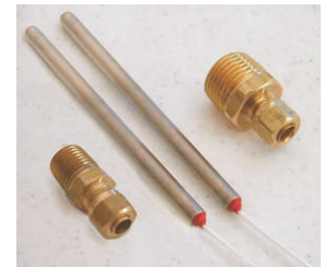
PRECISION BTU MEASURING TEMPERATURE SENSORS (+/-0.2F) #SOLR-TS13-02 IMRS 2-SENSOR 1/4"NPT FTG 2.5"L #SOLR-TS23-02 IMRS 2-SENSOR 1/2"NPT FTG 2.5"L #SOLR-TS14-02 IMRS 2-SENSOR 1/4"NPT FTG 4"L #SOLR-TS24-02 IMRS 2-SENSOR 1/2"NPT FTG 4"L #SOLR-TS15-02 IMRS 2-SENSOR 1/4"NPT FTG 8"L #SOLR-TS25-02 IMRS 2-SENSOR 1/2"NPT FTG 8"L
